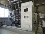
Water purification system with electrical resin regenerator
