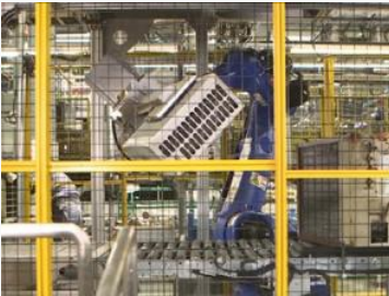
Machine to turn over air conditioner outdoor units at PETECK
