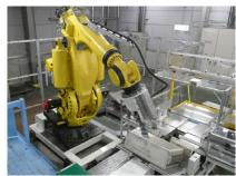
Automatic Dismantling System for Used Appliances
